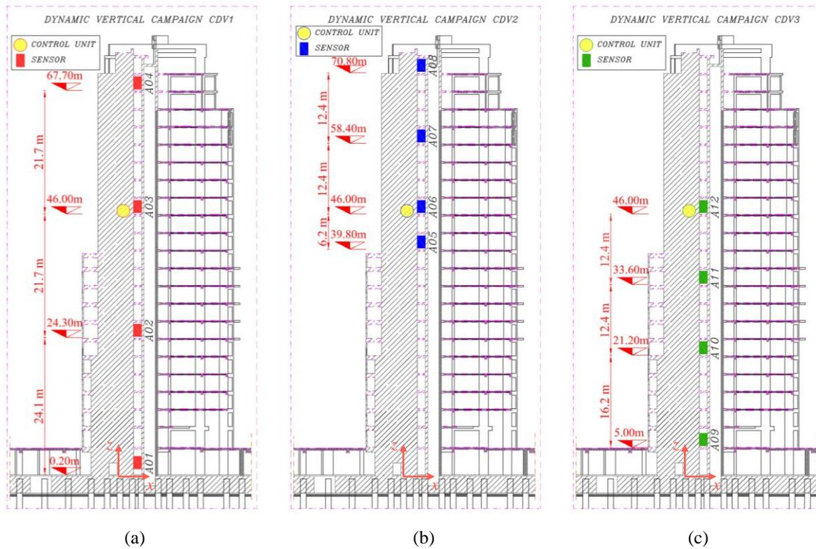
**Figure 2.** (a) Vertical campaign along the entire height CDV1; (b) Upper levels vertical campaign CDV2; (c) Lower levels vertical campaign CDV3.
