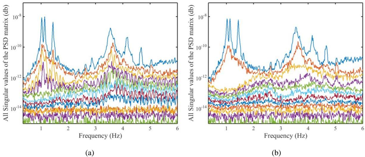
**Figure 3.** (a) Singular Value spectrum for channels not synchronised; (b) Singular Value spectrum for synchronised tracks.
