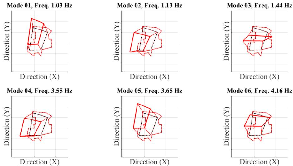
**Figure 9.** In-plane mode shapes from CDH at the lift level n°12 (top view).
