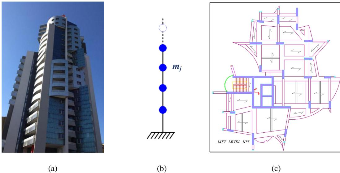
**Figure 1.** (a) Multi-storey building analysed; (b) Vertical rod model, fixed ended at the base; (c) Pillars disposition on the representative storey n°7.
