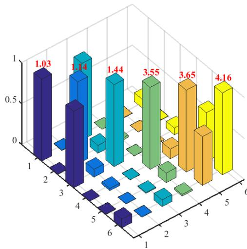
**Figure 8.** MAC of the assembled vertical modes.
