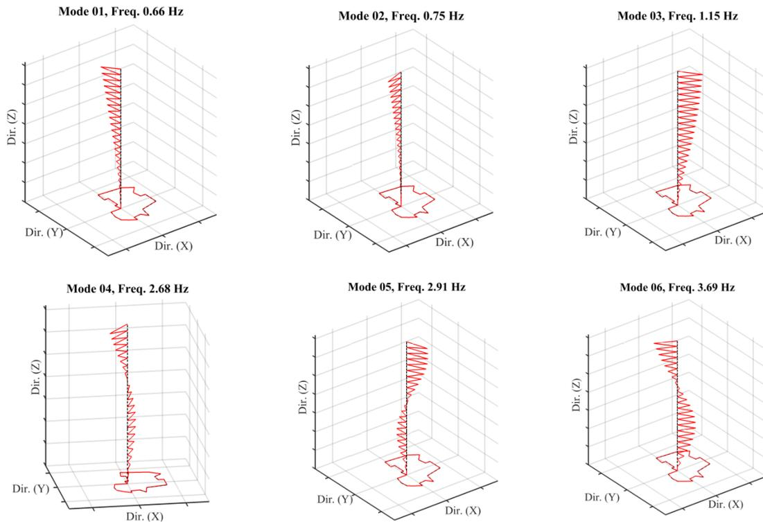
**Figure 11.** Vertical mode shapes simulated with the FEM model.
