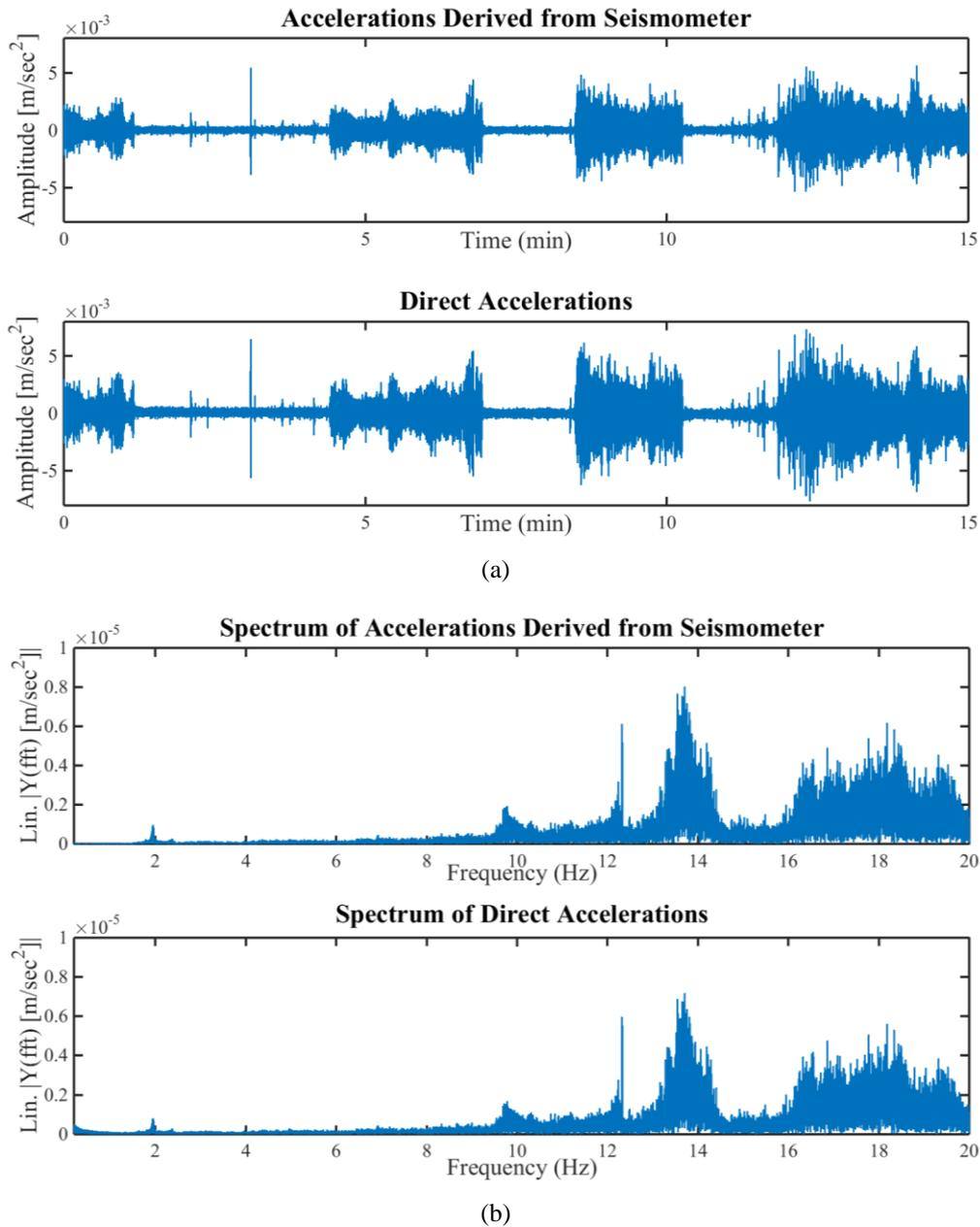
**Figure 4.** (a) Accelerations in time, comparison between derived and direct signals; (b) Spectral comparison between derived and direct accelerations.
