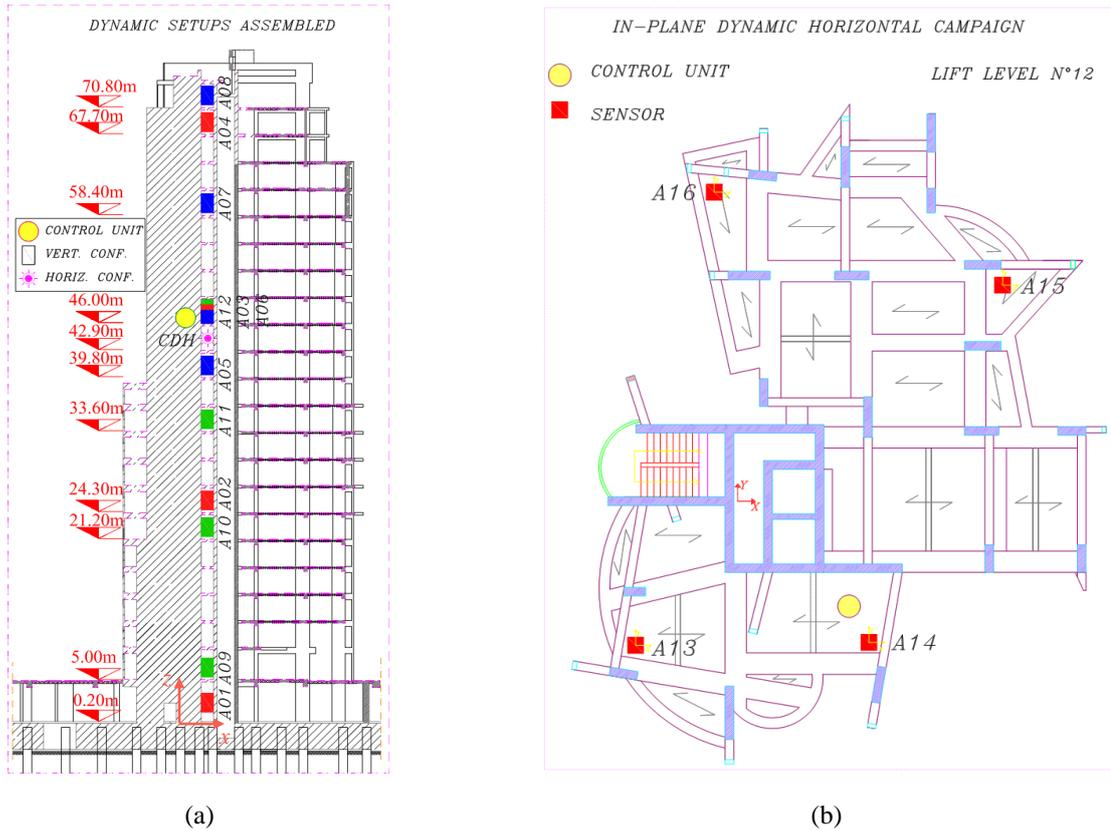
**Figure 5.** (a) All dynamic setups assembled; (b) Horizontal campaign on Level n°12.
