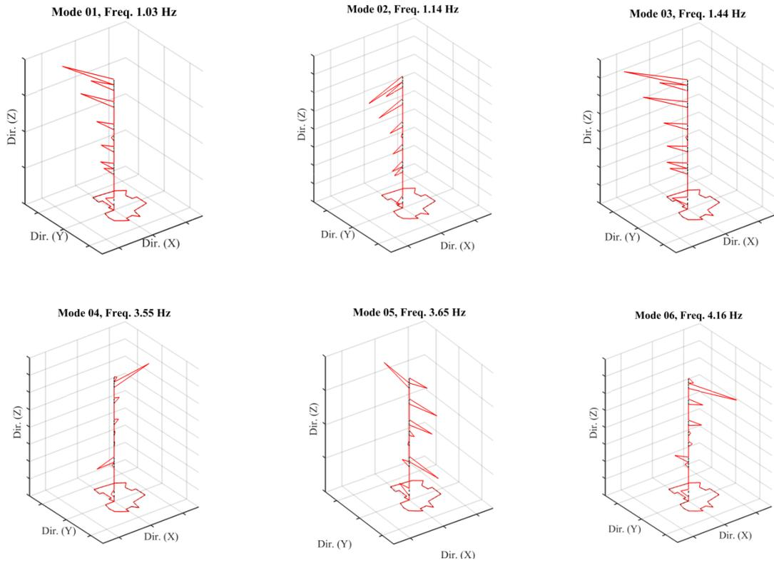
**Figure 7.** Vertical modes assembled in an overall setup for the first six experimental mode shapes.
