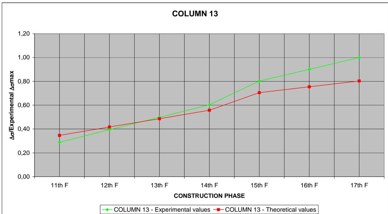
**FIG. 6** COLUMN 13: THEORETICAL AND EXPERIMENTAL STRESS INCREMENTS IN DIFFERENT CONSTRUCTION PHASES
