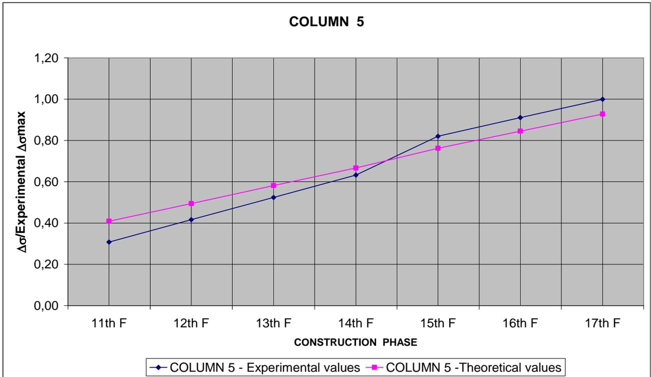
**FIG. 6** COLUMN 5: THEORETICAL AND EXPERIMENTAL STRESS INCREMENTS IN DIFFERENT CONSTRUCTION PHASES
