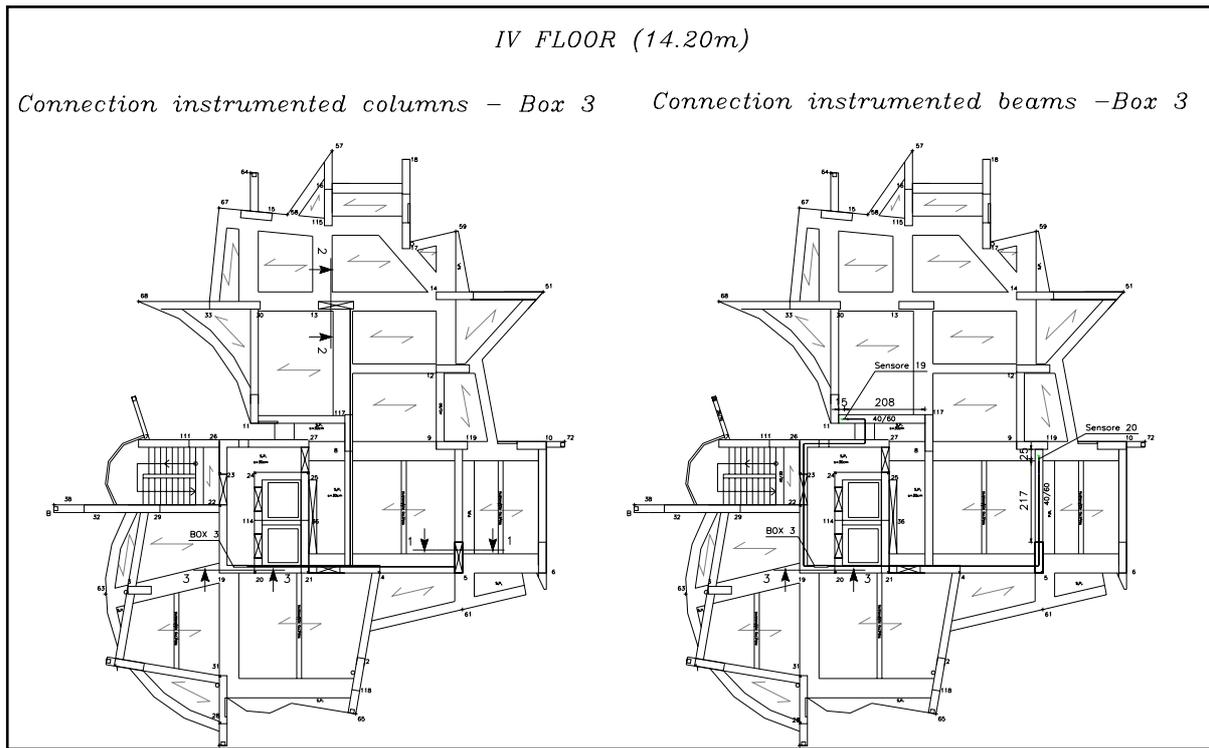
**FIG. 5 IV FLOOR - MONITORED BEAMS AND COLUMNS**
